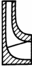
Fig. 2. Single suction, horizontal or vertical centrifugal pumps with narrow port impellers have low capacities and deliver high heads. Specific speed range is 500 to 1000.
