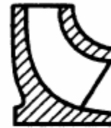
Fig. 4 Single or multistage, and single (illustrated) and double suction, Francis-type impellers, operating in volute or diffuser type casings produce medium to high capacity at medium to low speeds. Specific speed range is 2000 to 4000.
