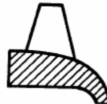
Fig. 6 Single or multistage pumps with mixed flow and propeller-type impellers have very high capacities and deliver very low heads. Specific speed range is 6000 to 10,000.
