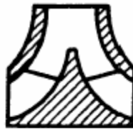
Fig. 3. Single or multistage, double (illustrated) and single suction, volute and diffuser design centrifugal pumps deliver medium capacity and medium heads. Specific speed range is 1000 to 2000.
